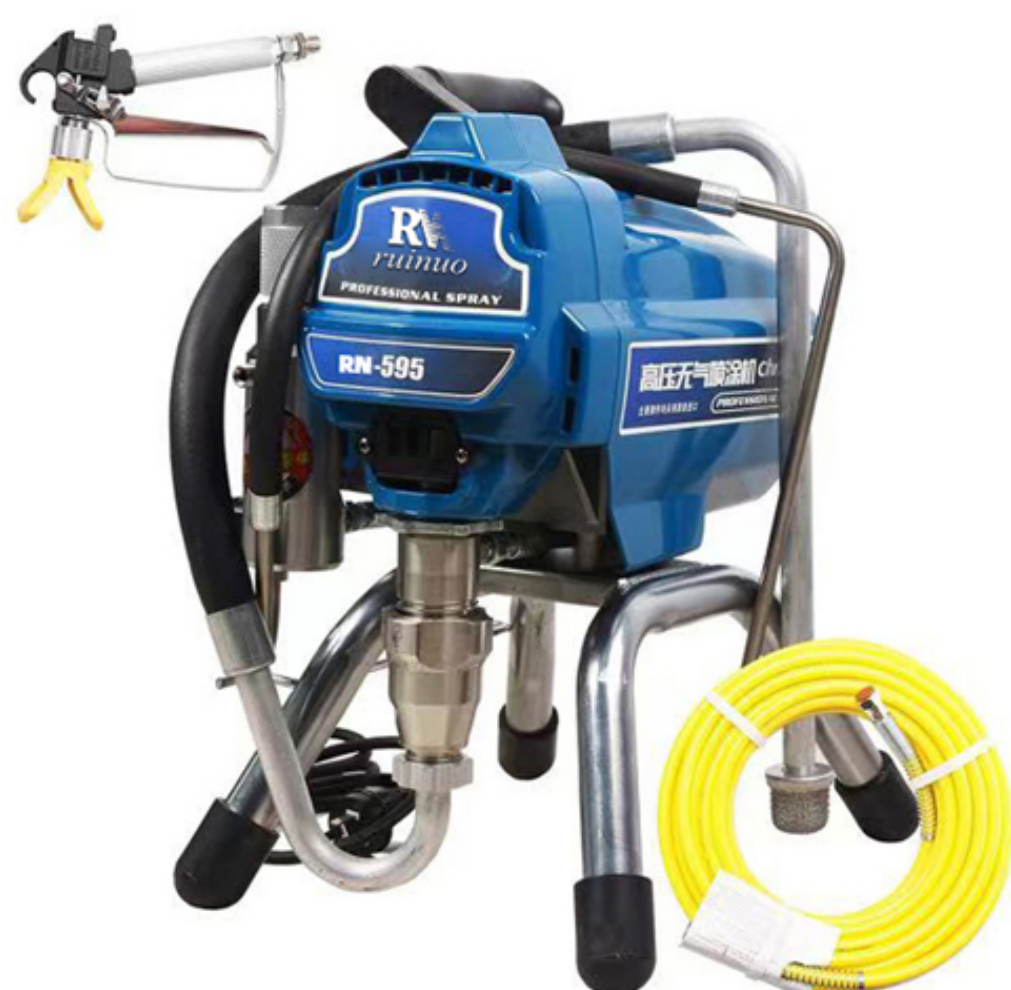
High perssure airless sprayer
